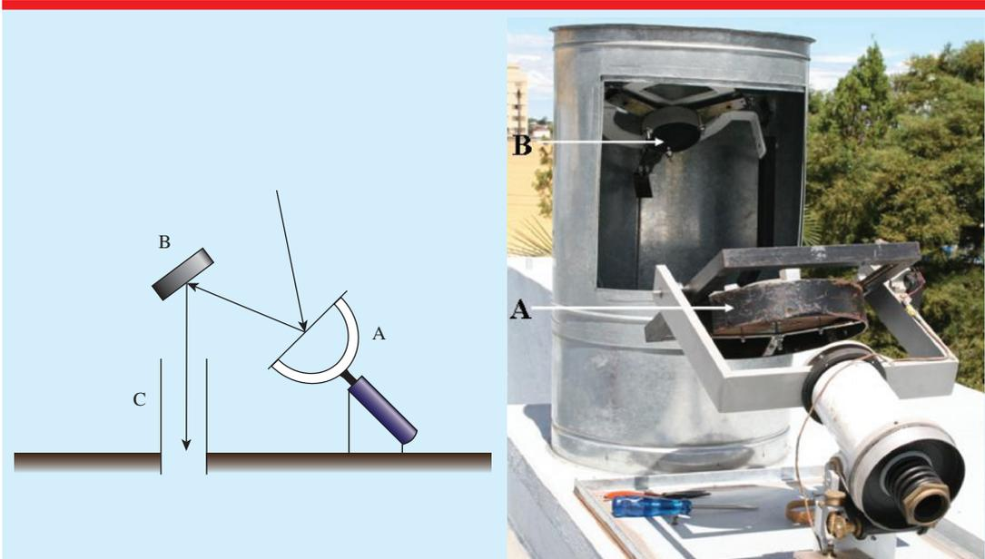
**Figure 1.** Left: diagram of a heliostat with movable primary mirror (A), fixed secondary mirror (B) and telescope (C). Right: image of the heliostat, where A is the primary mirror and B is the secondary mirror.
