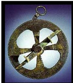
Used to determine the latitude of a ship at sea by measuring the altitude of the Sun or star, the mariner's Astrolabe was popular in the late 15th and early 16th Centuries.
